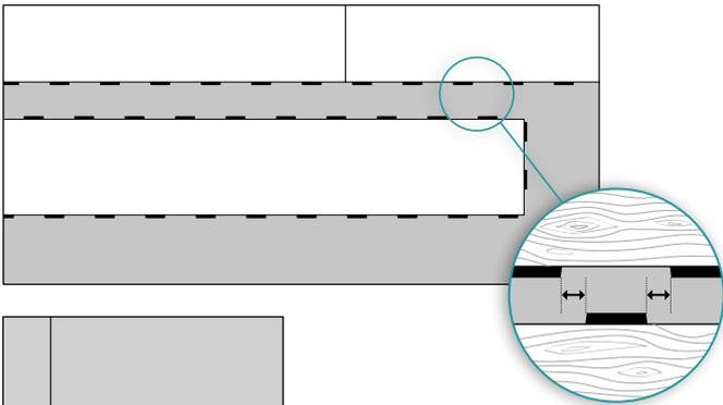
The click elements of the new row, need to be positioned, exactly in the middle of two locks of the previous row.
