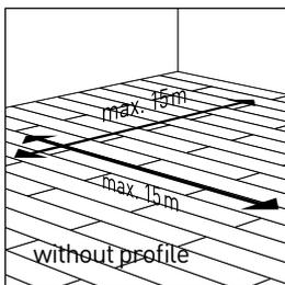
The largest recommended installation area is 15 x 15 m. An expansion profile must be used in door openings, and/or if the area is longer/wider than 15 m.
