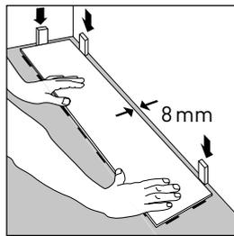
Measure the room to create a balanced layout. By measuring, you will be able to determine if the first row needs to be cut. The first and last rows should not be less than 5 cm wide.
