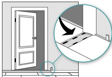
For doormouldings, lay a panel face down next to the door moulding. Saw the panel, then slide the plank under the moulding.
