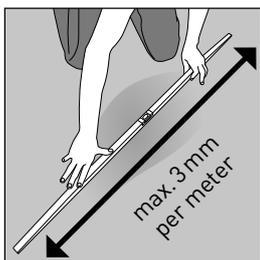
Make sure floor level deviation is a maximum of 3 mm per m, and 2 mm per 20 cm. If these margins are exceeded, the subfloor must be evened out with a suitable filler or levelling compound, and a check must be carried out to determine if a sealer is needed.
