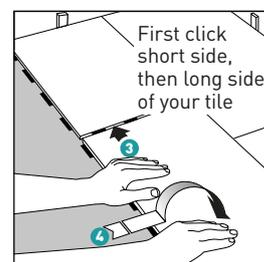
Always ensure that the short end joints are staggered by a minimum of 20 cm (= 2 click elements) when you start the next row. Use the leftover piece from the previous row as the first piece of the next row, provided that this piece is at least 20 cm long. In order to find a connection with the locking tabs of the previous row, it may be necessary to cut off an extra part of the leftover piece.
