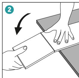
Do not use a hammer to put planks together. Cut boards with a Stanley knife, decor side up.
