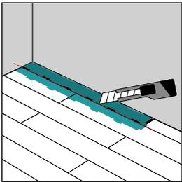
To install the last row, position a loose panel exactly on top of the last laid. Place another panel upside down up to the wall and mark the panel underneath. Cut the marked panel to size and fit in place.
