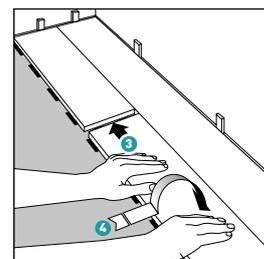
Always ensure that the short end joints are staggered by a minimum of 30 cm (= 3 click elements) when you start the next row. Use the leftover piece from the previous row as the first piece of the next row, provided that this piece is at least 30 cm long. In order to find a connection with the locking tabs of the previous row, it may be necessary to cut off an extra part of the leftover piece.
