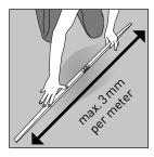
Remove all traces of plaster, paint, glue, oil, grease, etc. The subfloor must be clean, flat, dry and stable. Remove textile floor coverings (such as carpet, needle felts, etc.) Remove all debris (including nails) and vacuum.
