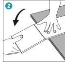
Do not use a hammer to put planks together. Cut boards with a Stanley knife, decor side up.
