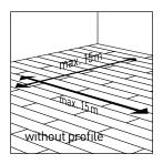
The largest recommended installation area is  $15 \times 15 \, \text{m}$ . An expansion profile must be used in door openings, and/or if the area is longer/wider than  $15 \, \text{m}$ .
