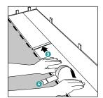
Always ensure that the short end joints are staggered by a minimum of 30 cm (= 3 click elements) when you start the next row. Use the leftover piece from the previous row as the first piece of the next row, provided that this piece is at least 30 cm long. In order to find a connection with the locking tabs of the previous row, it may be necessary to cut off an extra part of the leftover piece.
